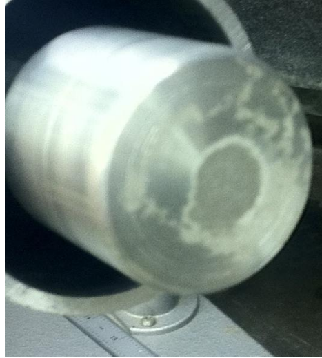
Figure 4.23: Damage Occurring on the Surface of the Electrode after Sustained Operation with High Delivered Power
